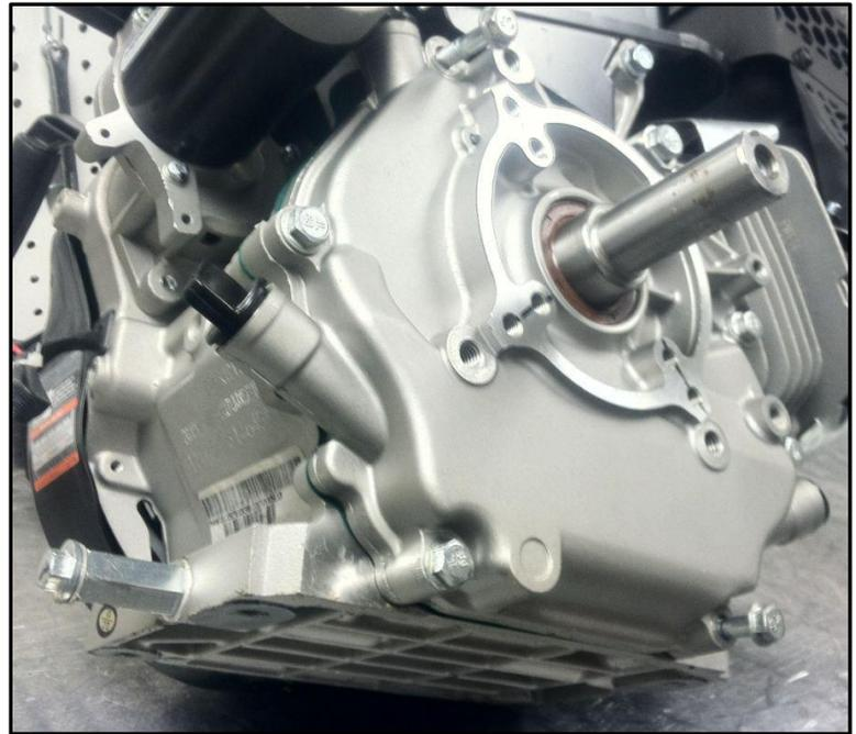
*Proper removal of PTO cover bolts; 414cc Snow King*
